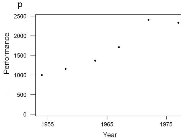
Figure 10 – Performance of tires incorporating mixed generations of tire cords
