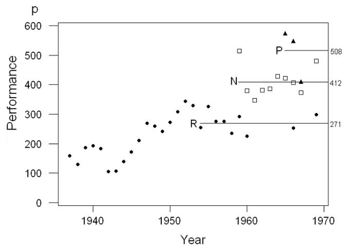
Figure 9 – Tire Cord Performance calculated from pPQ
